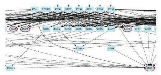
Fig. 4. Excerpt of a call dependency diagram of the CalculateInterest COBOL programs
