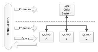
Fig. 7: Example of variability due to CQRS
